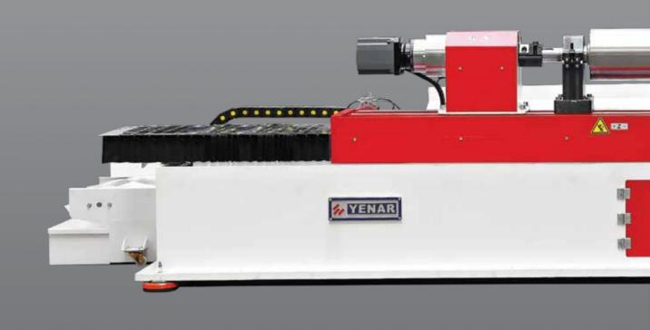
Once the fluting cycle is designed as simple as possible to avoid any skills. The cutting depth is automatically calculated according to diagrams such as angles, land, flutes on circumference or per cm by the machine. The grinding cycle is also very simple as fluting cycle. You need to enter total cut and just choose one of the pre defined grinding shape. (Cylindrical, chamfer or camber).
